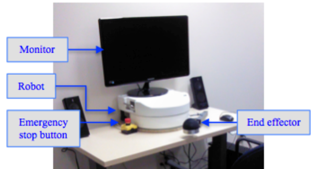
Figure 1: Image of the upper limb rehabilitation robot with a monitor to display a Graphical User Interface
